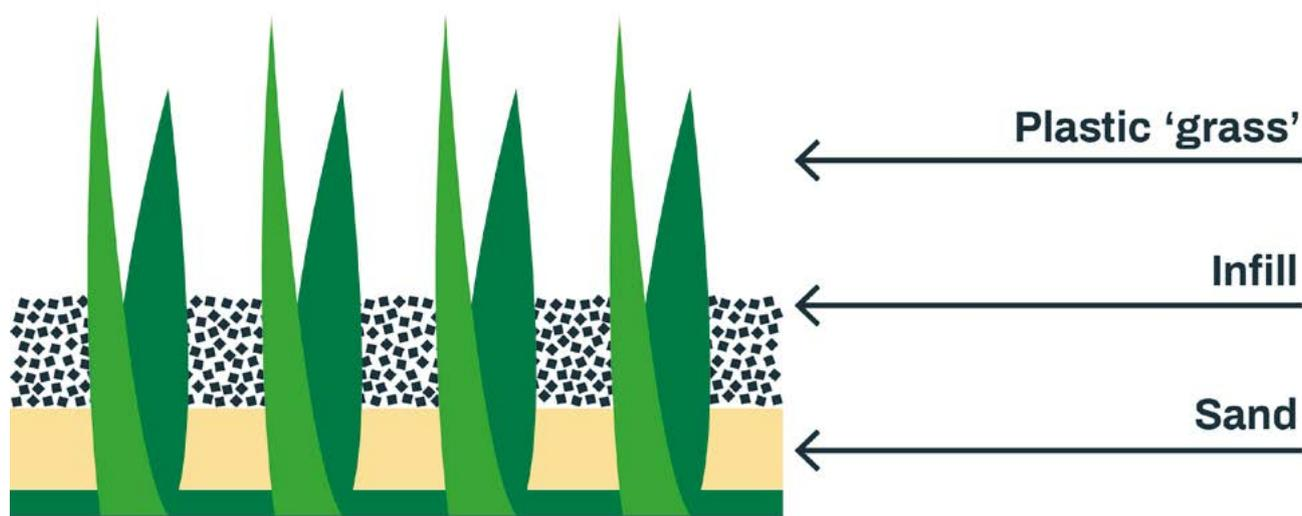
Many artificial sports pitches use third generation (3G) technology, which means fine granules are added as a **performance infill** to make a more comfortable playing surface. Although alternative options are available, the vast majority<sup>2</sup> of pitches in Scotland still use microplastic as infill. The most common type is 'rubber crumb' from old vehicle tyres: a synthetic microplastic known as Styrene Butadiene Rubber (SBR).
